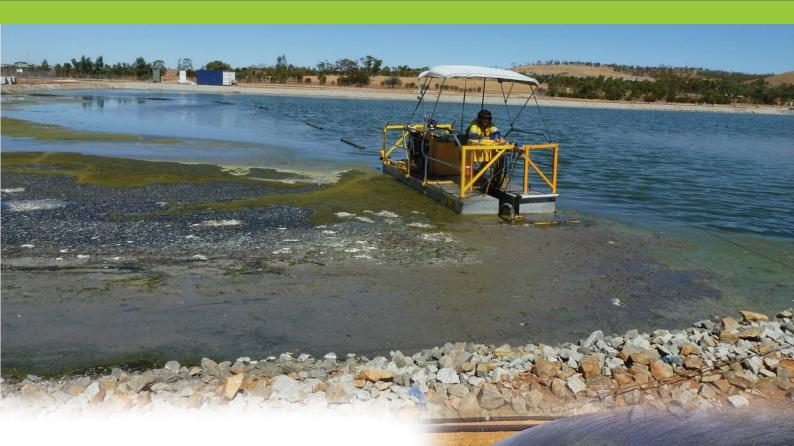
The GeoPro Microdredger and Desludging Tubes ensure the sediment removal is performed in a very controlled, cost effective way, using low energy, passive technology. We specialise in projects which demand a high level of expertise and close client and stake holder consultation. Because the GeoPro Microdredger is launched from our purpose built tilting trailer and is towed by a regular 4x4, we can access ponds and sensitive wetlands not usually accessible to larger machinery.
