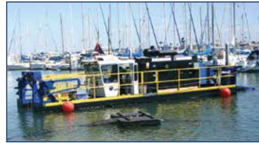
A Model 5012 HP removes sand from a large marina in California.
