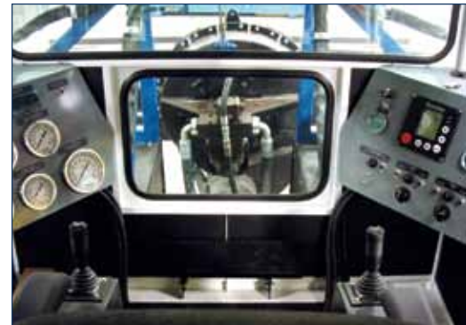
All Versi-Dredge® models come standard with joystick controls and oversized gauges for ease of operation.
