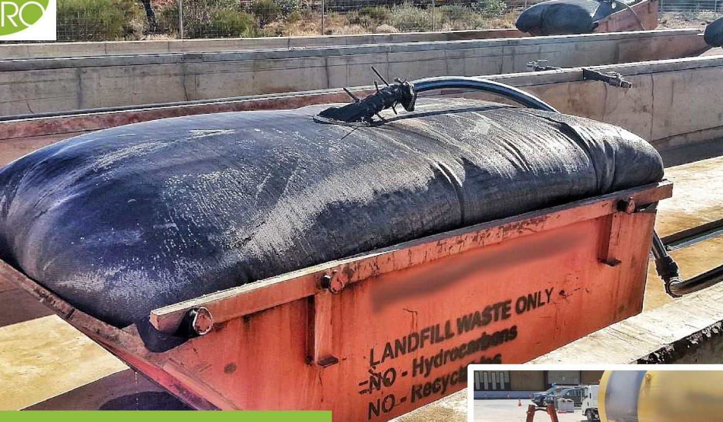
GeoPro Cubic Bags and frames are a very convenient and effective solids dewatering solution. They are ideally suited to smaller dewatering requirements for civil, mining, agricultural and industrial applications. The slurry is pumped or gravity fed into the cubic bags where with the aid of a polymer, solids flocculate and settle in the bag while the clear filtrate permeates through the geotextile membrane. Its compact size makes them maneuverable and easy to work with.
