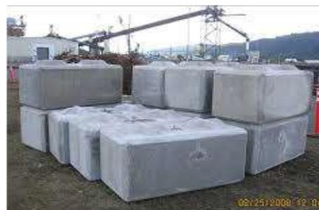
Large concrete blocks are a good choice for soft bottom lagoons as they will settle into the sediment. When using concrete blocks, the buoyancy of the concrete needs to be taken into account. This means a factor of approximately 10 must be taken into account to generate the required holding strength.
