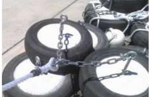
The holding strength required from the anchors will depend upon the operating conditions. In the case where large anchoring forces are required and it is impractical to deposit large and heavy anchors, multiple smaller anchors can be used to generate a similar anchoring weight. Ideally, anchors are placed (embedded where possible) in new ponds prior to filling.
